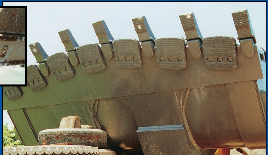
Esco V81VX tips – used in tight clay overburden removal.
