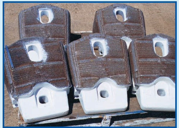
RIGHT: Esco 130 series adapters – A.R.M* Hardfaced on the top and both sides – often achieve over 5 times the wear life of the standard item.
