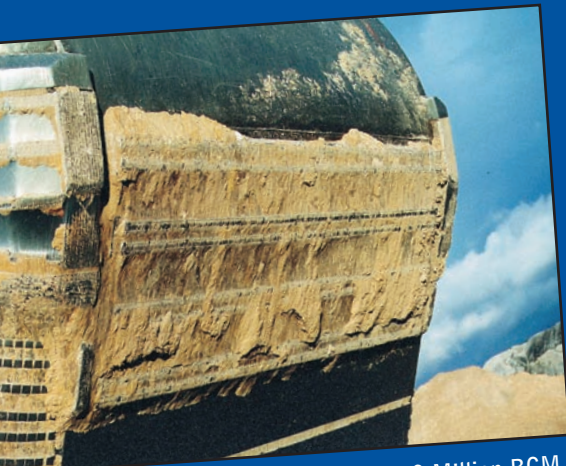
Dragline Bucket Heel Package after 1.0 Million BCM (usually 40mm Bis 80 only lasted 1.3 Million before holes appeared in the floor).
