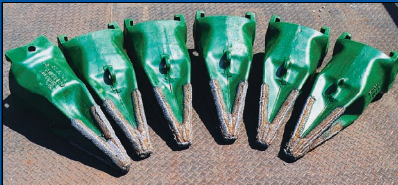
Esco V81VX tips – used in tight clay overburden removal.
