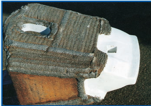
BEFORE: 130 series Dragline adapter prior to an A.R.M* rebuild.
