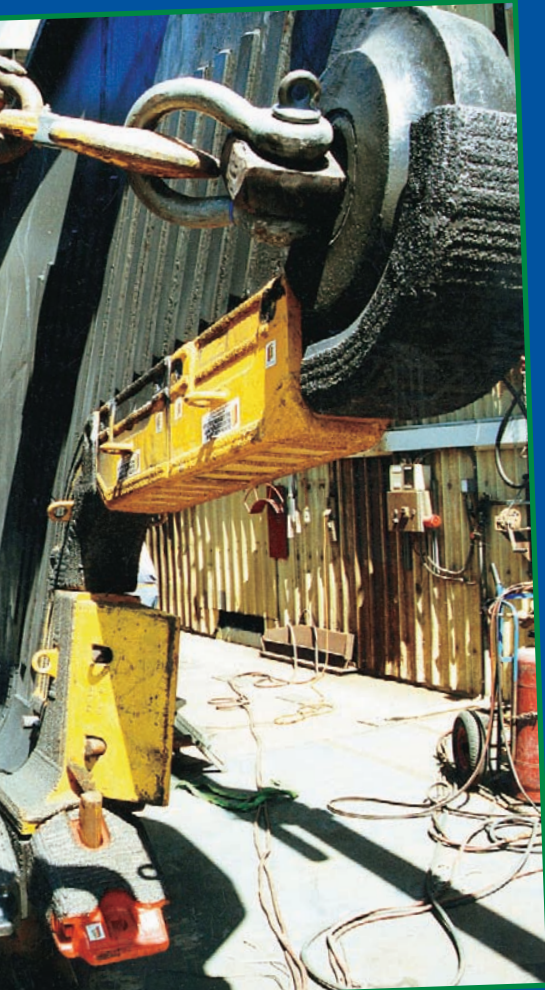
Dragline Bucket Jaw Shrouds A.R.M* Hardfaced.
