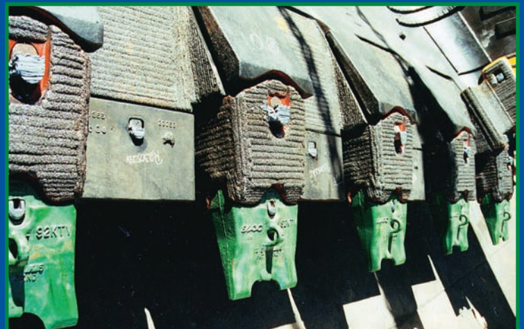
P&H Dragline Bucket Lip Shrouds A.R.M* Hardfaced.
