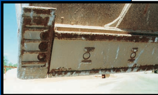
Esco V81VX tips – used in tight clay overburden removal.
